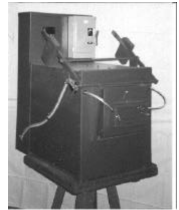
U-75B-D Furnace with Rear Mounted Control Panel
